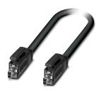
Patch cable, type: IEC 63171-2, degree of protection: IP20, cable length: 1 m, number of positions: 2, 1 Gbps, connection method: Crimp connection, connection cross section: AWG 22- 22, Single Pair Ethernet
