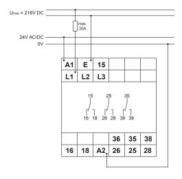
Measuring range 288V DC, supply voltage 230V AC
