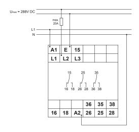
Measuring range 360V DC, supply voltage 24V AC/DC
