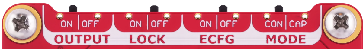
Figure 4-1. Configuration Slide Switches
