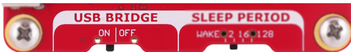
Figure 3-3. USB Bridge Slide Switch
