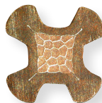
Indenter Crimp Cross-Section Across Axis Figure 2
