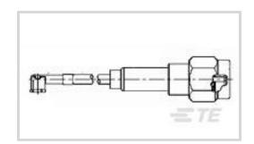
Cable Assembly Type: OSMT to SMA
