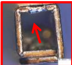
Terminal damage from header pin
