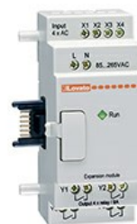
Micro PLC expansion module, 4 analog inputs 0... 10VDC/0...20mA LRE04AD024 24VDC n° 4 analog
