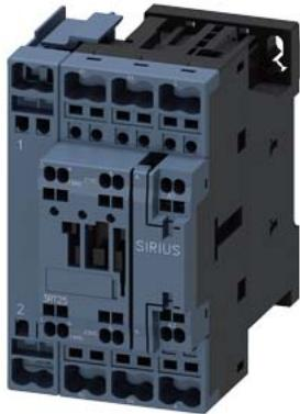
power contactor, AC-3, 25 A, 11 kW / 400 V, 4-pole, 24 V AC, 50/60 Hz, main contacts: 2 NO + 2 NC, auxiliary contacts: 1 NO + 1 NC, spring-loaded terminal, size: S0
