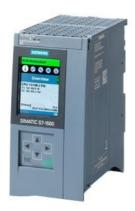
SIPLUS S7-1500 CPU 1515R-2 PN based on 6ES7515-2RN03-0AB0 with conformal coating -40...+70 °C . central processing unit with work memory 1 MB for program and 4.5 MB for data, 1st interface: PROFINET RT with 2-port switch, 2nd interface: PROFINET, SIMATIC Memory Card required
