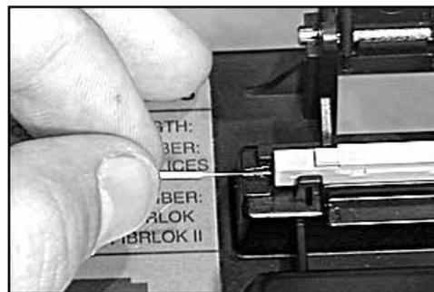
4.6 Gently push the second fiber in small increments straight through the alignment guide into the fiber entry port. As the coating of the second fiber enters the fiber entry port, watch for the bow in the first fiber to increase. This occurs when the end face of the second fiber contacts the first fiber and pushes the first fiber slightly back out of the splice. Continue gently pushing the second fiber until it meets resistance.
