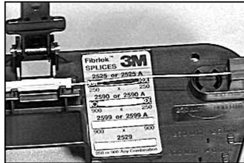
4.4 Prepare second fiber (strip, clean and cleave) as described in Section 3.
