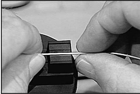
4.2 Grasp the coated fiber about .25 inches (6 mm) from the bare glass and move the fiber end onto the fiber alignment guide on the assembly tool such that the end is resting on the alignment guide outside of the splice.
