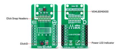
The VEML6046X00 sensor provides distinct peak sensitivity values at 600nm for red, 550nm for green, 470nm for blue, and 820nm for infrared, enabling accurate RGBIR detection in both natural and artificial light environments. With an impressive ambient light detection range of 0 to 176,000 lux and a fine resolution of just 0.0053 lux, this sensor excels in capturing subtle changes in lighting for dynamic system response.
