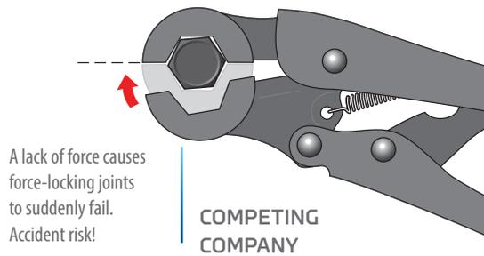
A lack of force causes force-locking joints to suddenly fail. Accident risk!
