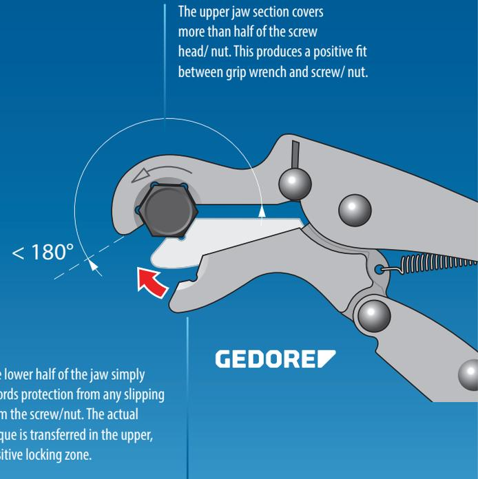
The upper jaw section covers more than half of the screw head/ nut. This produces a positive fit between grip wrench and screw/ nut.
