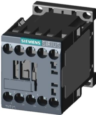
power contactor, AC-3, 12 A, 5.5 kW / 400 V, 4-pole, 42 V AC, 50/60 Hz, main contacts: 2 NO + 2 NC, screw terminal, size: S00
