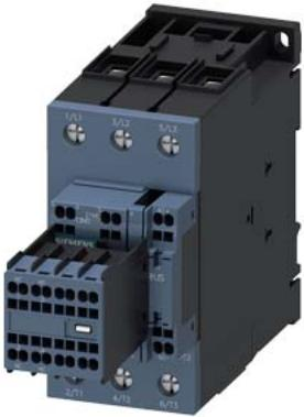
traction contactor, AC-3e/AC-3, 65 A, 30 kW / 400 V, 3-pole, 24 V DC, 0.7-1.25\* Uc, solid-state operating mechanism, with integrated varistor, auxiliary contacts: 2 NO + 2 NC, main circuit: screw terminal, control and auxiliary circuit: spring-loaded terminal, frame size: S2, removable auxiliary switch
