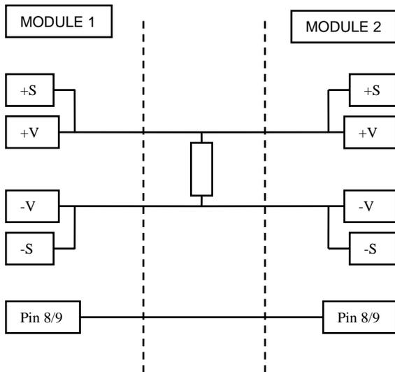
**Parallel for increased current : Not redundant.**
