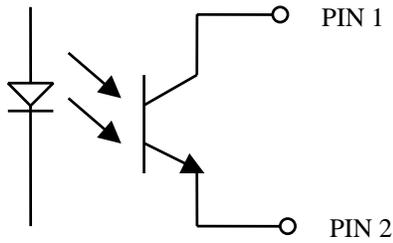
This provides an opto-isolated output which provides a minimum of 5mS warning before loss of output power due to either loss of AC input or over temperature of the converter.
