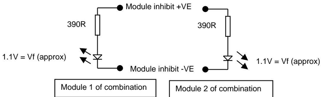
Both options need to have the opto isolated diodes connected in parallel.
