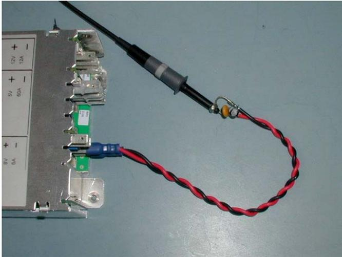
Noise from a switching power supply is made up of two distinct elements "ripple" and "high frequency". "Ripple" noise is the variation at the switching frequency of the supply. "High frequency" noise is superimposed on top of the "ripple" and results in a typical waveform as below.
