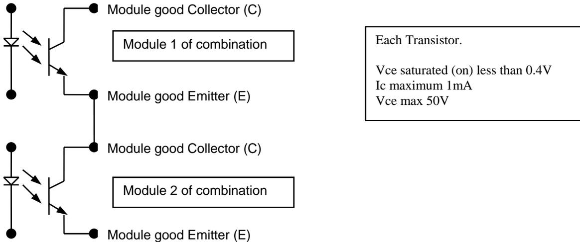
Both transistors ON = Module combination GOOD.
