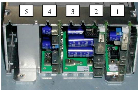
The picture shows a typical Vega configuration with faston output connections :-
