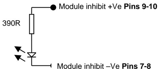
Internal to the module inhibit/enable is a 390ohm 1/8W resistor and the diode of an opto-coupler.
