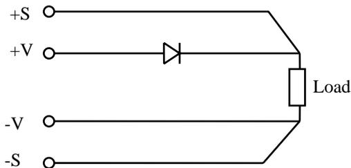
Do NOT fit components (resistor, inductor or diode) into remote sense lines. This will make the system unstable.
