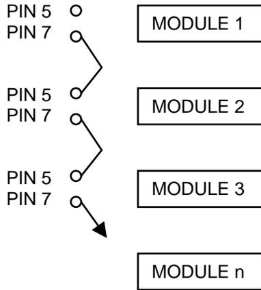
All the PIN 5 and PIN 7 perform the same function and are linked internally in the module.
