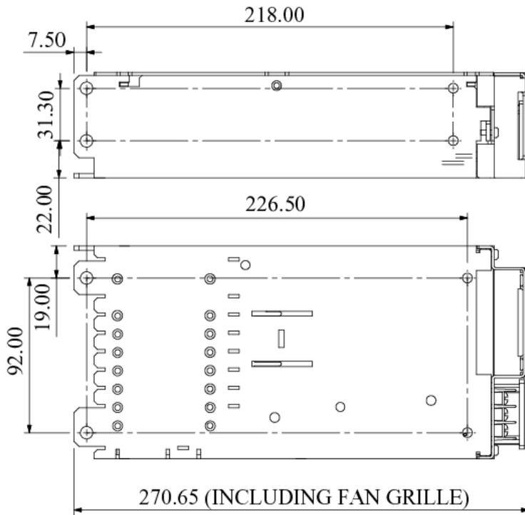
Access to screw terminals may be gained by removing terminal cover.
