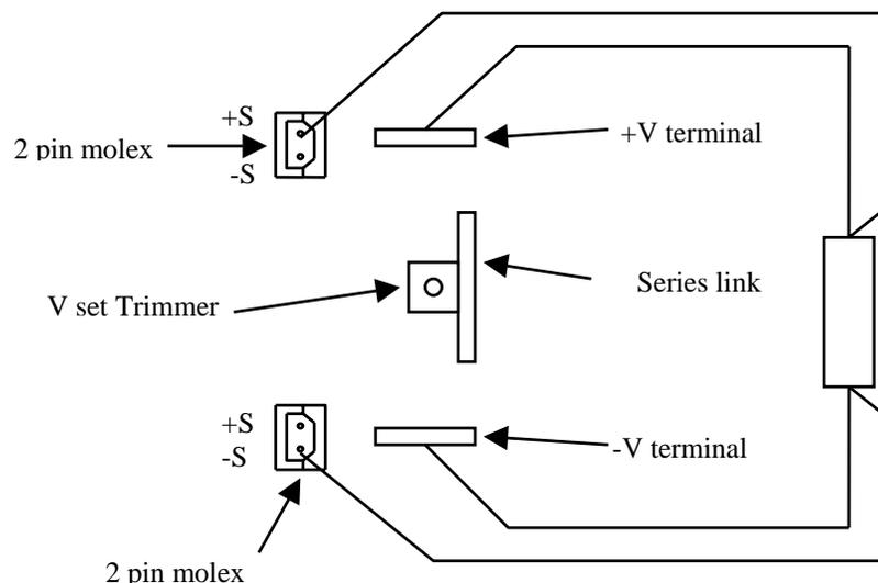
Connect +S from the top 2pin molex connector to +V of the load.
