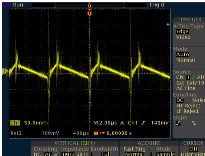
The term PARD means "Periodic and Random Deviation" and is a measure of the TOTAL noise (ie high frequency noise + ripple) quoted as peak to peak. This is the figure quoted in the specifications of each module.
