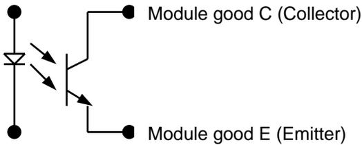
Module is GOOD when output voltage is between 90%(+/-5%) and 110%(+/-5%) of its factory set voltage.
