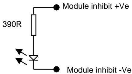
Internal to the module inhibit is a 390ohm 1/8W resistor and the diode of an opto-coupler.
