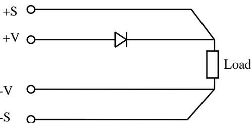
Do not fit components (resistor, inductor or diode) into remote sense lines. This could make the system unstable.
