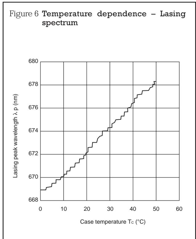
Temperature also affects the laser diode by altering the threshold current. An increase of 25°C increases the threshold current and therefore the supply current of the laser module by about 10mA. Operating at the higher current reduces the life of the diode and therefore every effort should be made to maintain the operating temperature of the laser module at the minimum practicable for the application.
