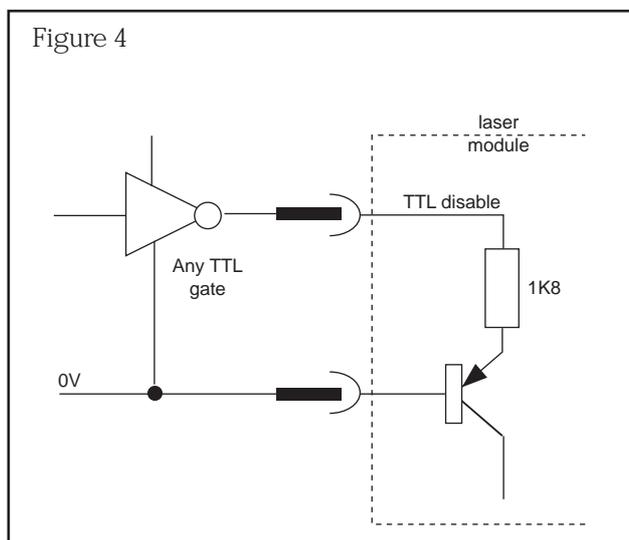
An input voltage above 4V will turn the laser off. When not in use, this input can be left floating or if preferred, connected to 0V.
