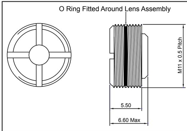
The collimating lens consists of a single element of high index glass with a laser quality anti-reflection coating on both surfaces. This design is simple yet highly efficient, producing very low divergence coupled with well defined spots of light at short, medium and long range.
