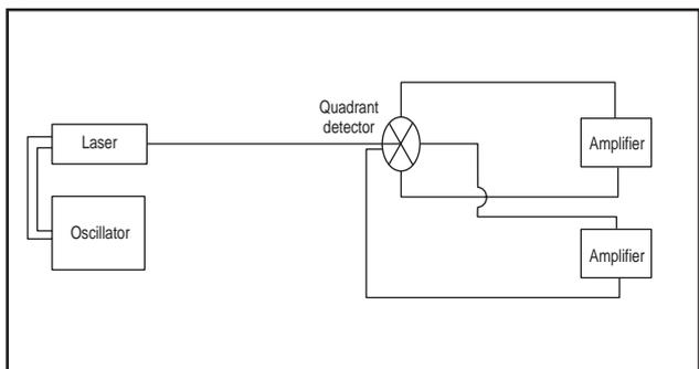
Two such systems used side by side on the item to be aligned not only give greater accuracy in the XY position, but also registers rotational errors. The spots of light from lasers 1 and 2 show not only vertical and horizontal position, but as the spot from laser 1 is below the centre of detector 1 and that from laser 2 is above the centre of detector 2, there is an element of rotation illustrated by the line joining the two spots.
