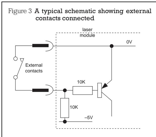
Any voltage applied to this input must not exceed +2.5V or be less than -5V.
