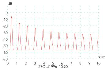
The spectrum analyser view uses a Fast Fourier Transform (FFT) to convert a set of samples taken at fixed time intervals into a distribution showing the amount of energy in each of a number of frequency bands up to a maximum frequency. The maximum frequency is half the frequency corresponding to the sampling rate.
