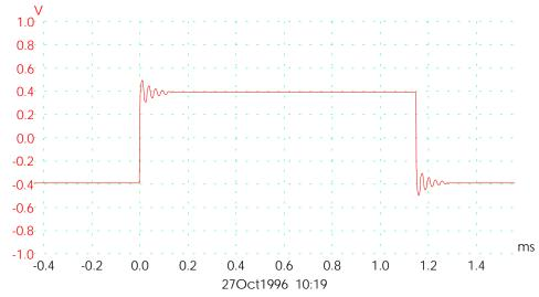
If the trigger event occurs only once, it is useful to be able to stop immediately after collecting the data for the trigger event. You can do this by checking the **Stop on trigger** option in the **Trigger dialog**, or by setting the trigger mode to **Single** in the sample bar.
