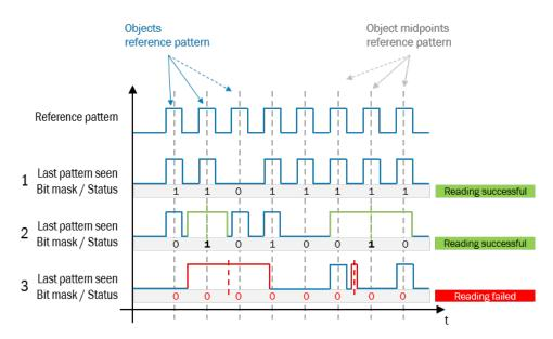
Figure 15: Midpoint evaluation (Direct object detection) signal schema
