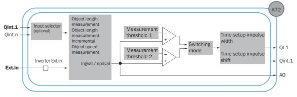
Figure 7: Logical principle of operation A72
