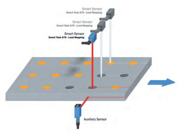
Figure 14: Workpiece carrier for Inverse object detection, width
