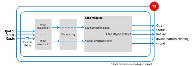
Figure 11: Logical principle of operation A75
