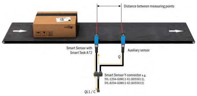
Figure 8: Wiring example for "Length" and "Speed" measurement modes
