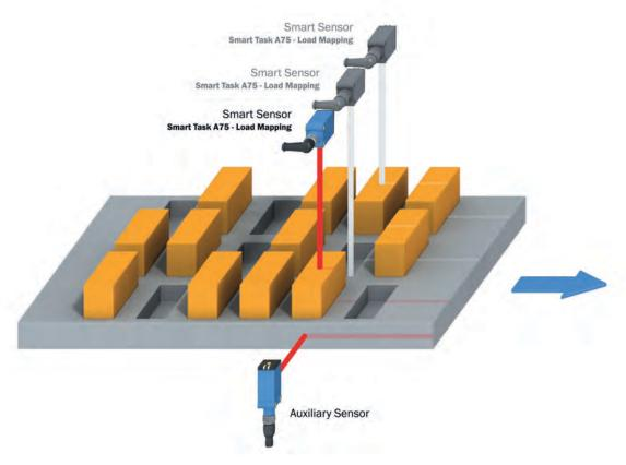
Figure 13: Workpiece carrier for Direct object detection, midpoint/width mode
