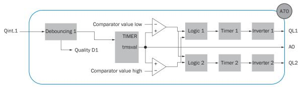
Figure 5: Logical principle of operation A70
