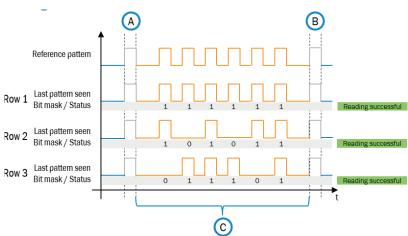
Figure 17: Workpiece carrier and the associated signal schema with pattern clipping: Two signal edges each at the beginning and end of the pattern are cut off and are not included in signal evaluation
