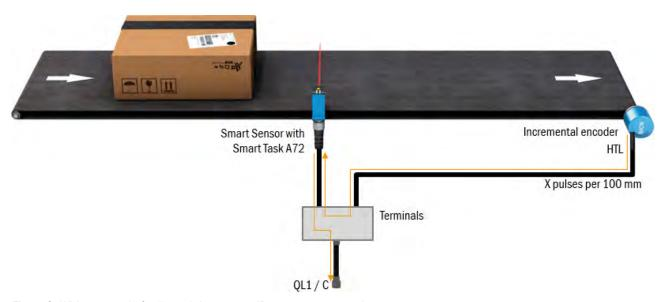
Figure 9: Wiring example for "Length incremental" measurement mode
