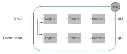
Figure 1: Logical principle of operation A00
