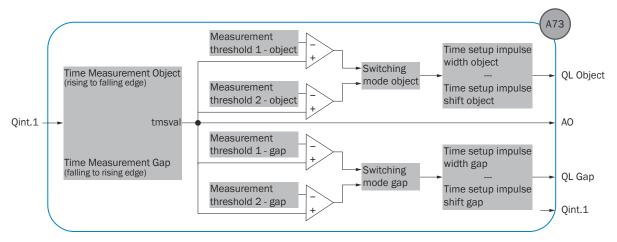
Figure 10: Logical principle of operation A73
