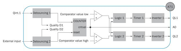
Figure 6: Logical principle of operation A71
