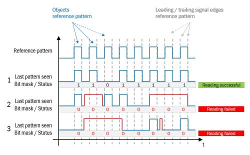
Figure 16: Width evaluation (direct object detection) signal schema
