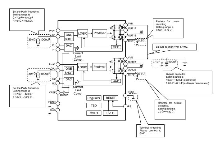
Fig.1 Block diagram & Application circuit diagram
