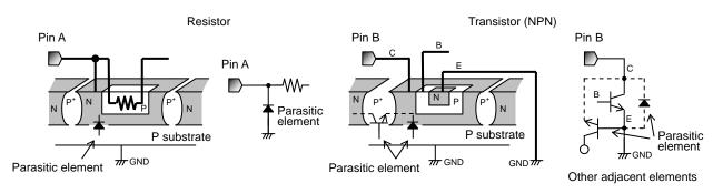
Fig.3 Pattern Diagram of Parasitic Element
