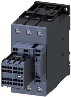
power contactor, AC-3e/AC-3, 80 A, 37 kW / 400 V, 3-pole, 110 V AC, 50 Hz, auxiliary contacts: 2 NO + 2 NC, main circuit: screw terminal, control and auxiliary circuit: spring-loaded terminal, size: S2, removable auxiliary switch
