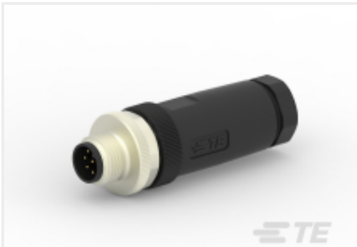
TE Part #T4111002081-000 M12,MALE,STRAIGHT,A CODE,8P, PG9,GOLD
