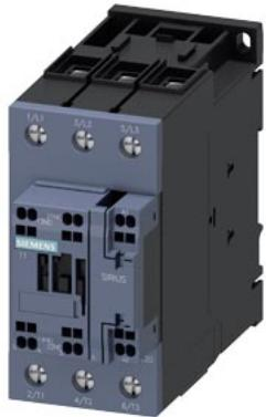
power contactor, AC-3e/AC-3, 65 A, 30 kW / 400 V, 3-pole, 83-155 V AC/DC, 50/60 Hz, with integrated varistor, auxiliary contacts: 1 NO + 1 NC, main circuit: screw terminal, control and auxiliary circuit: spring-loaded terminal, size: S2,
