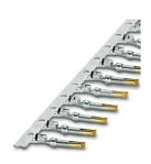
Crimp contact, Socket, rolled, Taped product, number of pieces per reel: 10000, contact diameter: 1 mm, crimp range:  $0.22~\text{mm}^2$  ...  $0.56~\text{mm}^2$ , Item is lead-free in accordance with RoHS II without Exemption 6c (Pb < 0.1~%)
