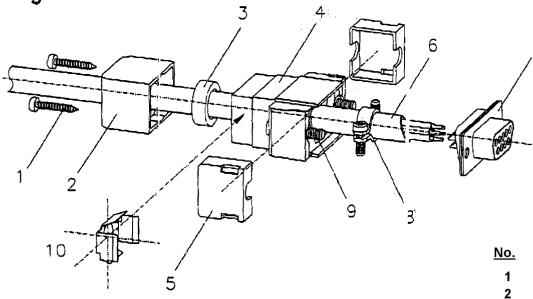
The black rubber gasket (3) is suitable for cable diameter 6,0 to 8,0 (0.234 to 0.310 ") with shell size 1, 2 and for cable diameter 8,0 to 10,5 (0.310 to 0.410 ") with shell size 3.
