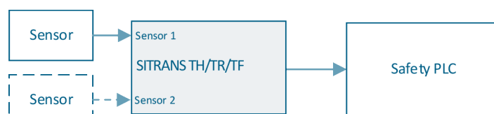
Figure 3 Single transmitter 1oo1 operation (SIL 2)
