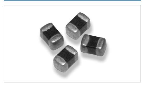
The P Series of multilayer beads is suitable for use in high current circuits due to its low dc resistance. It can match power lines to a maximum of 6 amps. The P series is available in 06:03 and 08:05 package sizes.
