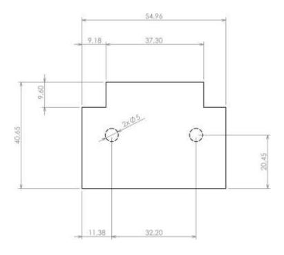
Dashed line shows outline of the mounting boss under PCB board Recommended mounting holes diameter ø3,5mm All dimensions are given within +/-0,5mm tolerance
