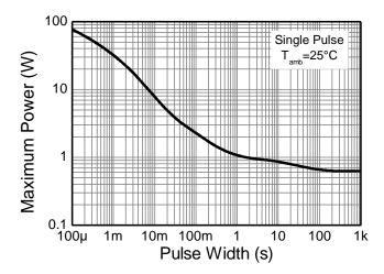
Figure 3. Pulse Power Dissipation
