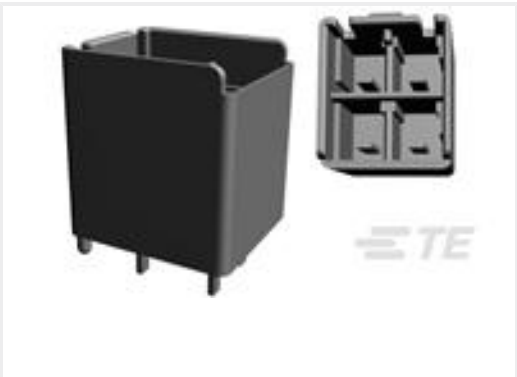
TE Part #1376386-2 5mm B-T-W Conn. 4P(2row) HDR A
