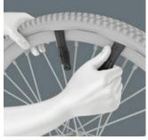
With the glass fibre reinforced plastic tyre levers, the tyres can be safely levered off the rim without damaging the rim. Lift off of the rim with one tyre lever, hook into a spoke and pull off the tyre with the second tyre lever. The two tyre levers can be clicked together and are therefore not lost individually.
