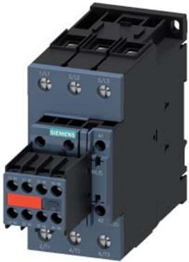
power contactor, AC-3e/AC-3, 41 A, 18.5 kW / 400 V, 3-pole, 230 V AC, 50/60 Hz, with plugged-in varistor, auxiliary contacts: 2 NO + 2 NC, screw terminal, size: S2, captive auxiliary switch
