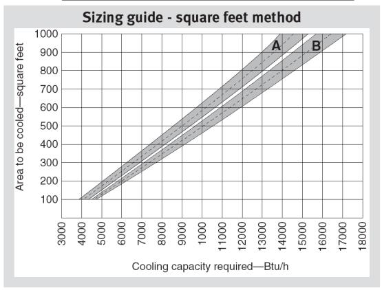
To calculate the approximate cooling required for a particular sized room the following rules can be applied:-
