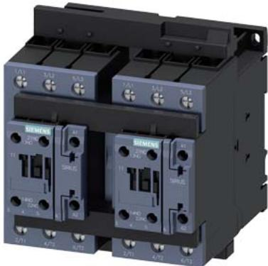
reversing contactor assembly, AC-3e/AC-3, 41 A, 18.5 kW / 400 V, 3-pole, 220 V AC, 50 Hz / 240 V, 60 Hz, screw terminal, electrical and mechanical interlock, auxiliary contacts: 2 x 1 NO
