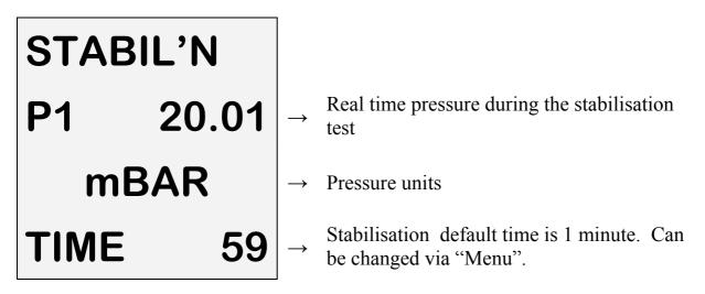
When stabilisation is complete press  $\leq$  to start the tightness test:
