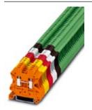
Feed-through terminal block, Connection method: Screw connection, Cross section: 0.14 mm<sup>2</sup> - 4 mm<sup>2</sup>, AWG: 26 - 12, Width: 5.2 mm, Color: red, Mounting type: NS 35/7,5, NS 35/15
