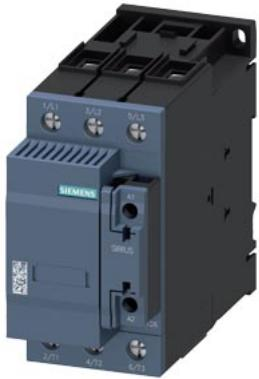
capacitor contactor, AC-6b 75 kVAr, / 400 V, 3-pole, 20-33 V AC/DC, 50/60 Hz, with integrated varistor, auxiliary contacts: 2 NC, screw terminal, size: S2
