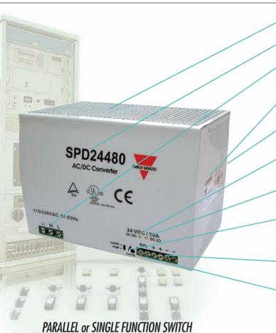
On the 240W and 480W versions the parallel/single function switch is a standard feature, on the 120W version it is available as an option. By setting this switch on the 'Parallel' position it is possible to connect up to three power supplies in parallel, in order to increase output power.
