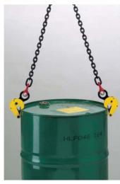
The DC500 drum clamp has been designed to lift and transport steel drums. If moving empty or sealed drums then one clamp is sufficient on its own. Should you be lifting an open full drum, then two clamps should be used with a two leg chain sling.
