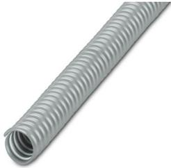
Protective hose, material: PVC, filament: PVC sheathed spring steel, UV-resistant: no, flexible, degree of protection: IP68, color: gray, inside diameter: 22 mm, Total length: 10 m
