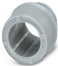
Cable protection end sleeve, material: PP, color: gray, flammability rating in acc. with UL 94: HB, inside diameter: 19.5 mm
