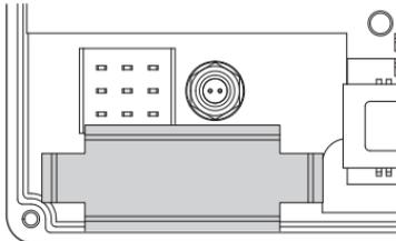
**11. Connect the battery and fit it into the battery space.**
