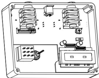
**6. Connect the Nutube circuit board and the main circuit board with harness A (52).**
