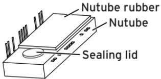
2. **Solder the Nutube (47) onto the side of the Nutube circuit board with the screen-printed surface.**
