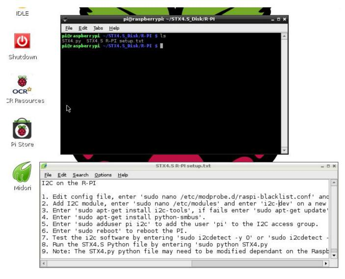
If you have not run any I<sup>2</sup>C connected devices on your Raspberry-Pi before then follow the procedure listed in the STX4.S R-PI setup.txt file. A reboot will be required to bring you back to desktop.
