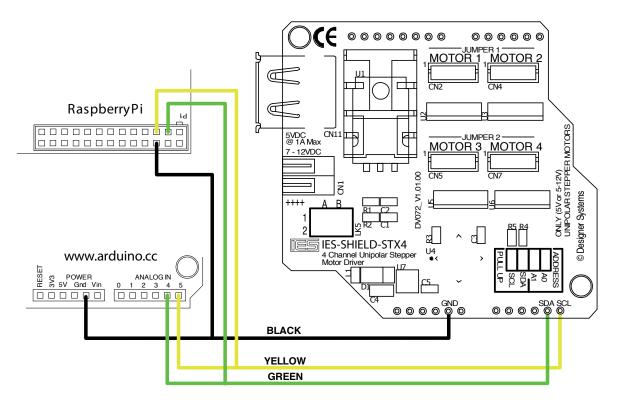
Connect a unipolar stepper motor (ie. DS-STMOT1) to the MOTOR 1 output, ensuring that the motor connection is pinned, from pin 1, /A, /B, A, B & V+. Ensure that the jumper links 1 & 2 are on position A. Connect a battery or power supply of 5 to 12Volts (depending on motor voltage) to the stepper power terminal block (ENSURE THAT POSITIVE ON THE BATTERY/POWER CONNECTS TO THE TERMINAL MARKED WITH ++++).
