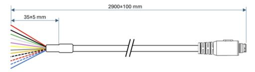
CA-MP-USB is a RS232 to USB cable that has the USB converter integrated at the end of the cable and consists of the following parts:
