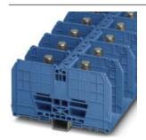
Bolt connection terminal block, Connection method: Bolt connection, Number of positions: 1, Cross section: 25 mm² - 300 mm², AWG: 4 - 600, Width: 54.8 mm, Color: blue, Mounting type: NS 35/7,5, NS 35/15
