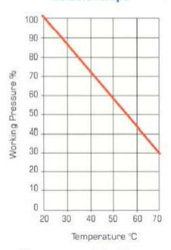
Max. recommended continuous working temperature = 60°C
