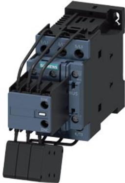
capacitor contactor, AC-6b 25 kVAr, / 400 V, 3-pole, 21-28 V AC/DC, 50/60 Hz, with integrated varistor, auxiliary contacts: 1 NO + 2 NC, screw terminal, size: S0
