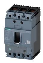
circuit breaker 3VA1 IEC frame 160 breaking capacity class N Icu=25kA @ 415V 3-pole, line protection TM240, ATAM, In=40A overload protection Ir=28A...40A short-circuit protection Ii=5...10 x In nut keeper kit
