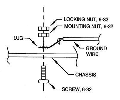
CHASSIS GROUND FOR SAFETY, USE ANY EMPTY HOLE ON THE POWER SUPPLY CHASSIS, PREFERABLY CLOSE TO THE TRANSFORMER INPUT FOR EASE OF WIRING.
