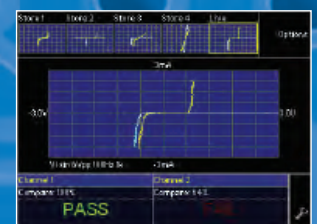
VI test with comparison against stored curve
