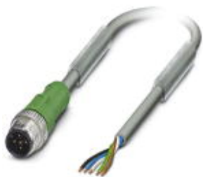
Sensor/Actuator cable, 5-position, PUR halogen-free, welding sputter-resistant, highly flexible, Gray RAL 7001, Plug straight M12, A-coded, on free cable end, Cable length: 10 m, for robots and drag chains
