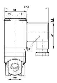
1+2 Solenoid\* and Socket turnable 4 x 90°
